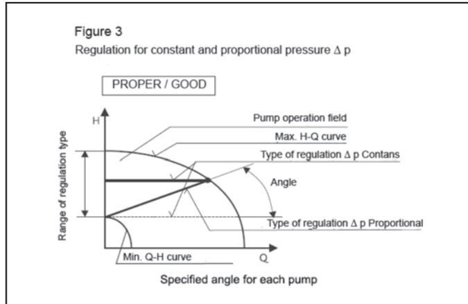
The proper selection of regulated pumps is shown in figures 3, 4 and 5. (Comparison of pump's characteristics determined by the design with actual technical characteristics of a particular pump).
