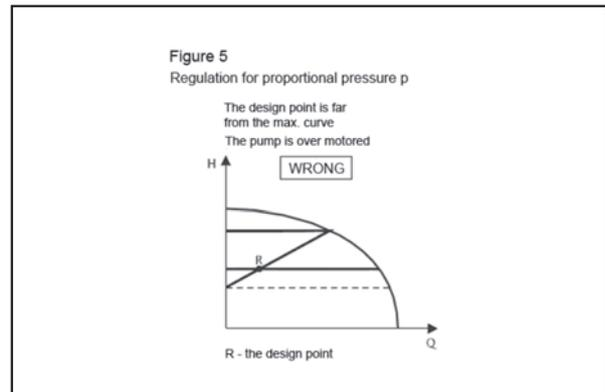
While using regulated pumps you can benefit from the operational field of a particular pump, which ranges from the minimal to the maximal Q-H curves. That is why such a regulation type is called stepless thermal regulation. The R design point should be located as close as possible to the functional max. Q-H curve.
